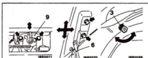
Adjustment of clearance around trunk lid and trunk lid striker engagement
