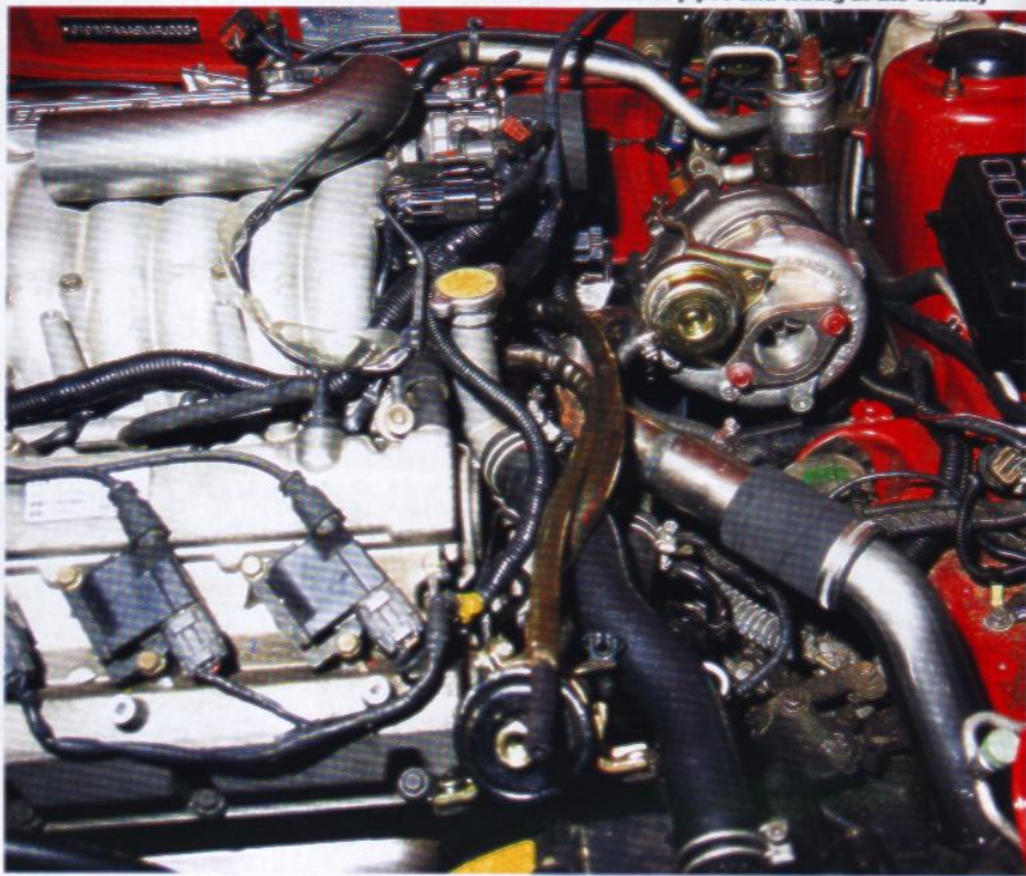
The small turbo was mounted above the bellhousing. Note the mass of pipes and wiring in the vicinity
