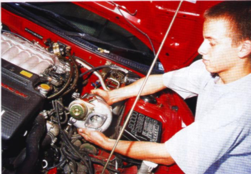
Some basic modelling showing where the turbocharger was going to have to sit
